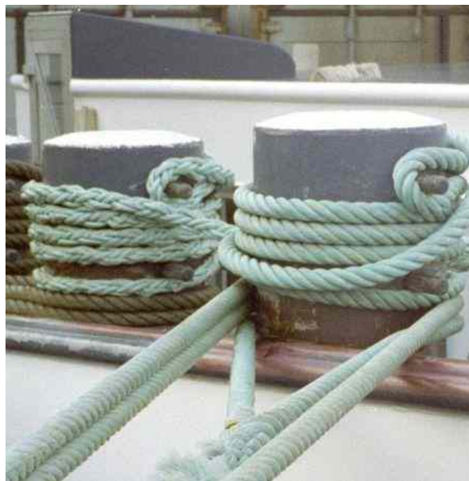
Figure 9: Synthetic lines used on inland navigation vessels
