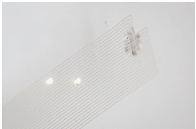
Figure 7. ( top ): overview image of a part of screen printed conductive patch and resulting via filling; ( bottom ): cross-section image of a filled via
