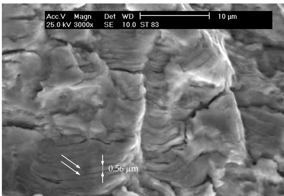
Figure 8: SEM micrograph of fatigue crack surface showing fatigue striations (magnification 3000x).
