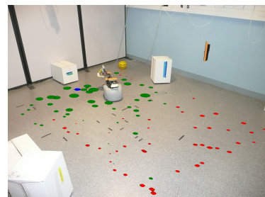
Fig. 3. Planning expert (red squares) vs. pre-trained taxon (green dots). The goal location is shown in blue. The robot has learned to choose the taxon (guiding) expert when close to the goal, while preferring the planning expert when the guiding fails farther away from the goal.
