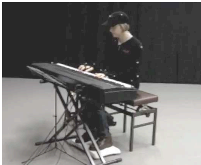
Figure 1. Experimental setup showing a performer playing, where MIDI and audio are recorded together with the pressure exerted by the feet using a Nintendo Wii Balance Board. The movement of the upper body was recorded using a MoCap system.
