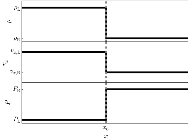
Figure 3.1: The general 1D Riemann problem. The primitive variables at the left and the right of x = x_0 are given at time t = 0 . We want to know what the values of the primitive variables are at an arbitrary later time t .
