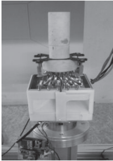
Figure 7.1: Photo of the custom designed cooling stage for \mu CT (De Schryver et al., 2014).
