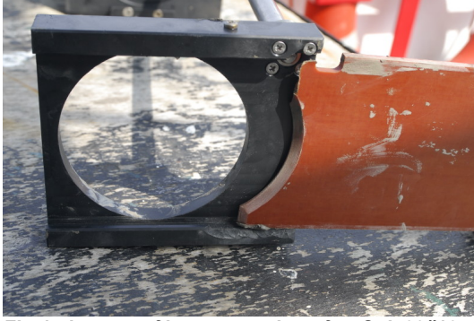
Fig 4: damage of bottom catcher after Gol700#10
