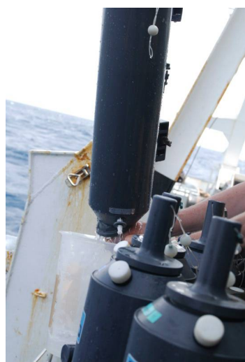
Fig 6: releasing the water from the Niskin bottle
