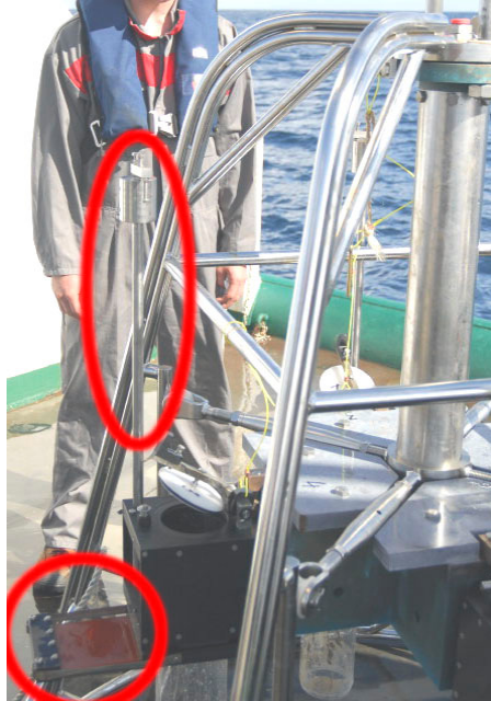
Fig 1: Fragile parts that are sticking out during deployment (bottom closer rod (upper) and bottom catcher (lower))
