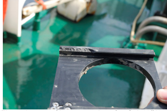
Fig 5: damage of bottom catcher after Gol700#10
