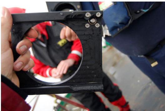
Fig 2: damage of bottom catcher after Gol700#2
