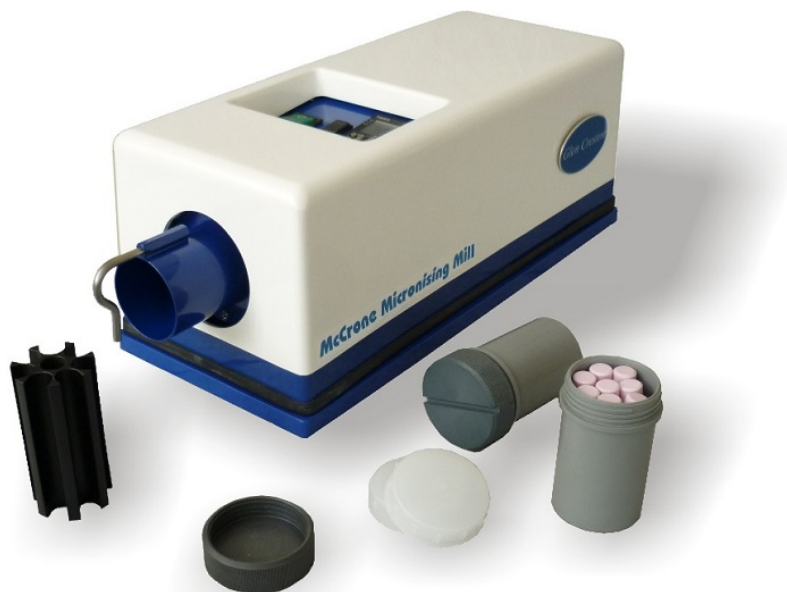
Figure 4.2: The McCrone ® micronizing mill device used in this study.
