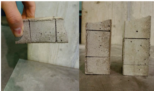
Figure 3.2 Specimens prior to splitting of the crack surface for bacteria extraction
