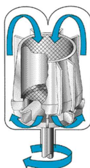
Figure 2-1. Cross sectional image showing the internal circulation in a Berty gas phase high pressure reactor.
