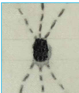
Figure 7.1 Fabricated PEDOT:PSS capacitor with three stainless steel yarn electrodes
