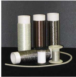
Figure 2.4 Metal clad fibers from AmberStrand®
