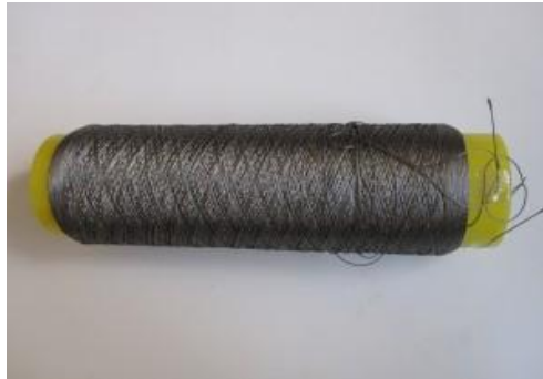
Figure 2.5. A bobbin of pure stainless steel filament yarns from BEKAERT BEKINOX ® VN
