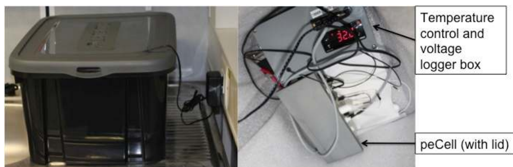
Figure 7.3 Insulated transportation box containing the peCell powered by the mains (left); the contents of the box (right).
