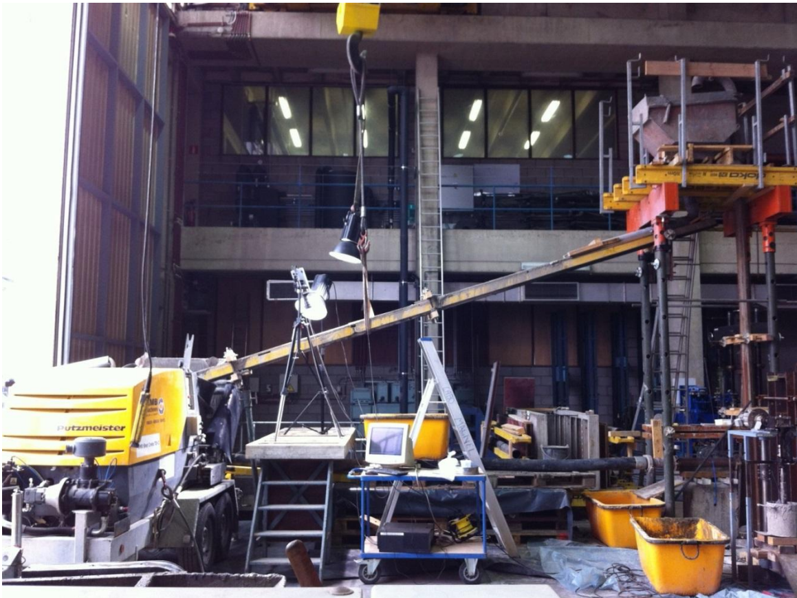
Figure 3-4 Circuit de pompage
