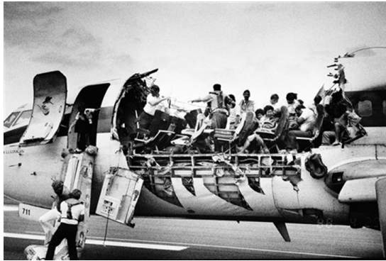
Figure 1.1: Aloha airline flight 243 accident [NSTB, 1989].
