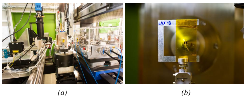
Figure 5.10: (a) Showing the general setup used at P06, Petra III (b) The chemically fixed worm, Lumbriculus variegatus mounted on kapton tape in front of the SLcam ® detectors 6:1 polycapillary lens.
