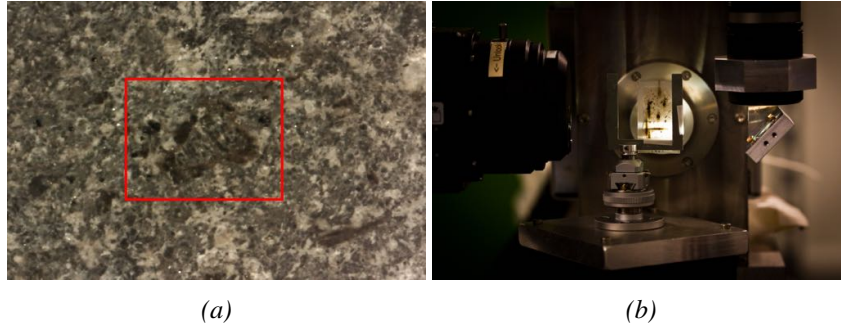
Figure 4.6: (a) Microscope image of the volcanic rock thin-section indicating in red the measurement area of about 1 mm ( H ) size. (b) (Middle) volcanic rock thin-section on a glass cover glass mounted in front of the SLCAM ® , (Right) pierced mirror of the in line beamline microscope, and (Left) the front of the PCO4000 detector at the P06 beamline, Petra III.
