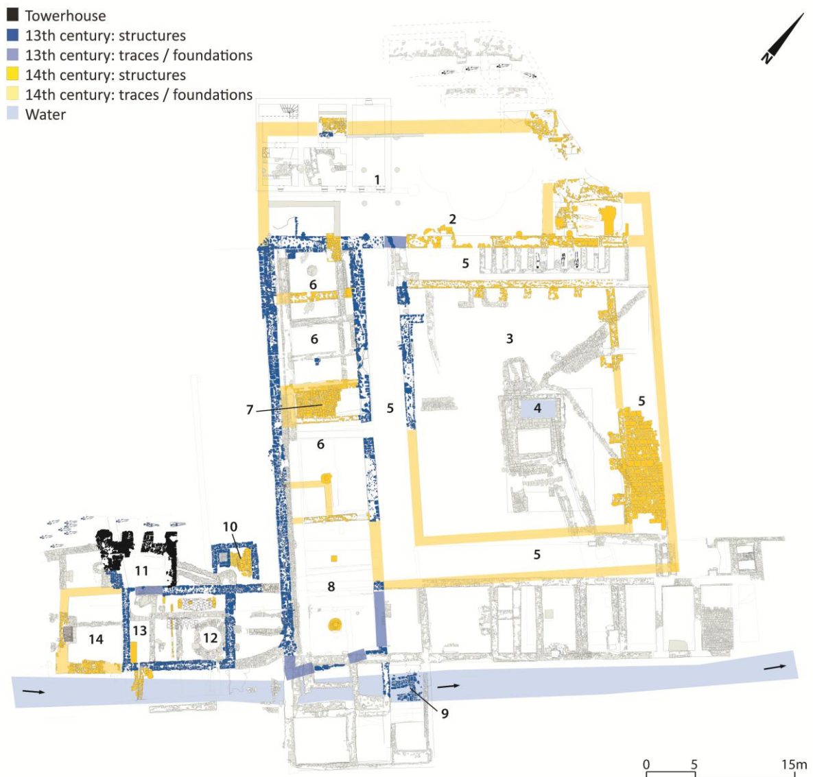
Figure 2—8 Clairefontaine II, ground level of the 14th century abbey: 1. church, 2. Saint Bernard's fountain, 3. Cloister garth, 4. Water basin, 5. ambulatory, 6. laysisters' wing, 7. pass way, 8. refectory, 9. latrines, 10. small kitchen, 11. fortified towerhouse, 12. kitchen, 13. annex of the kitchen with water basin, 14. annex of the kitchen (Davy Herremans, topography Dominique Bossicard, ©SPW-Dpat)
