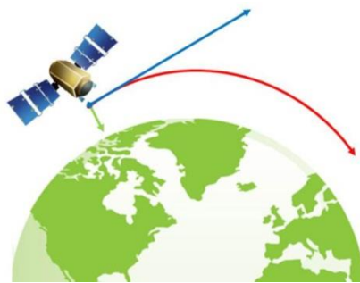
Figure 1: Scheme representing the gravitational force (green arrow) and propulsion force (blue arrow) which both act on satellites to generate the satellite orbit (red arrow). (Drawn by G. Pani)
