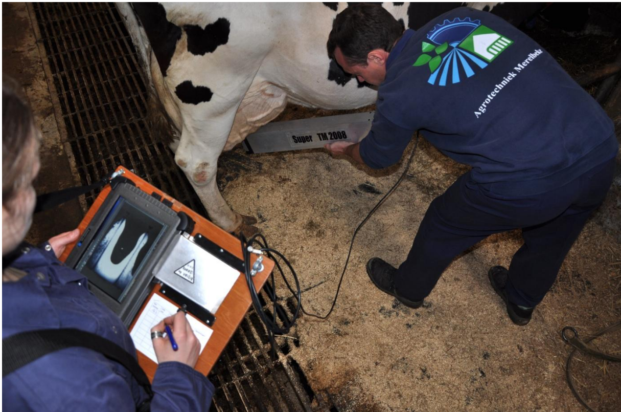
Figure 4. Teat measurements using the 2D vision-based measuring device in a tie stall.
