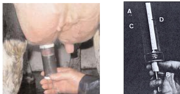
Figure 6. Transparent open-ended tube with graduated scale (A) without piston (Source: Gleeson et al., 2002) and (B) with piston (Source: Bakken, 1981)
