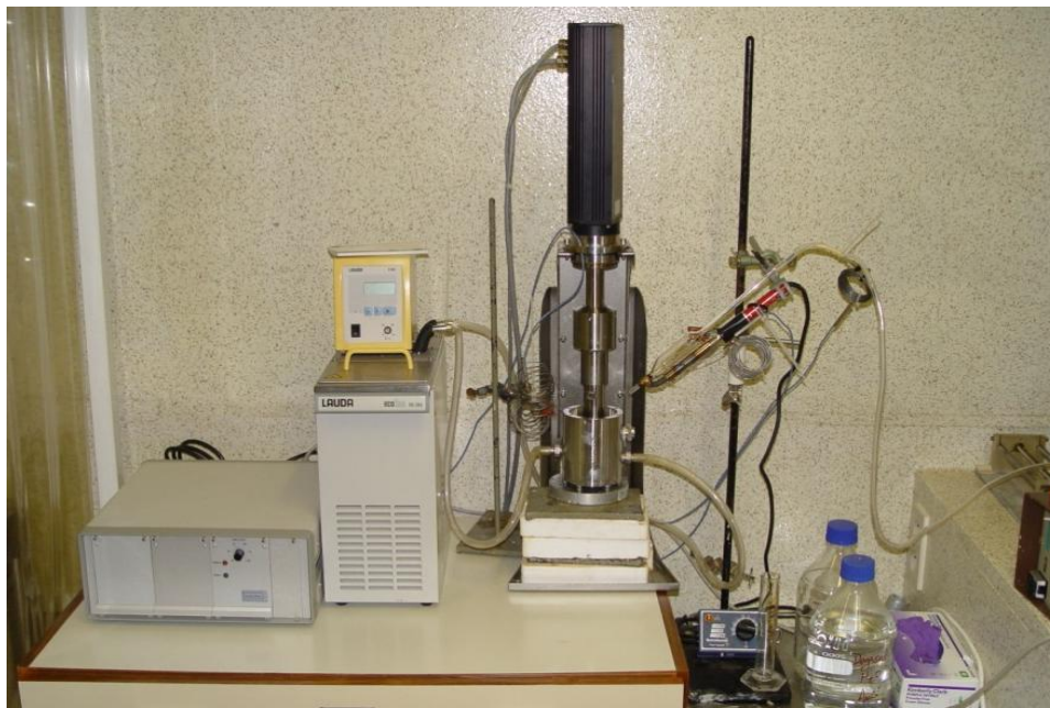
Figure 5. Photograph of the experimental ultrasonic melt crystallization set-up.
