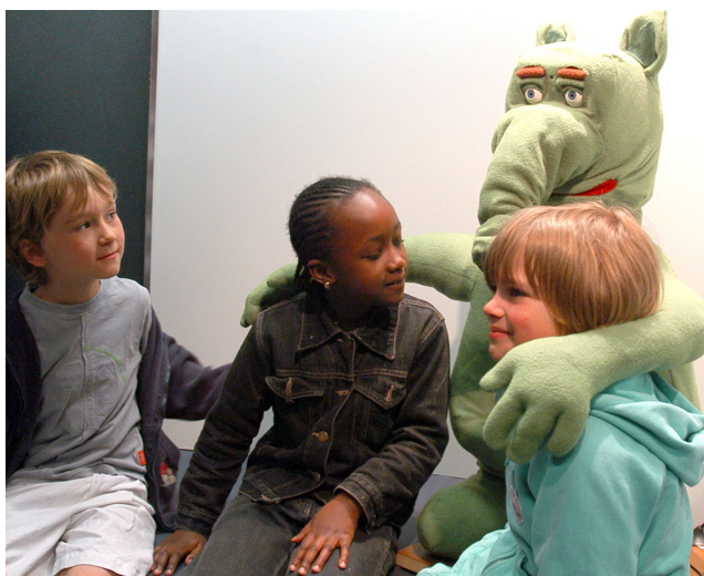
Figure 3.9: The prototype of the huggable robot Probo interacting with children.
