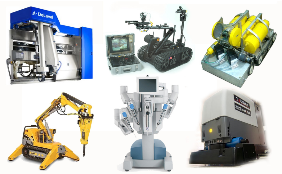
Figure 2.2: Examples of professional service robots for; milking, defense and exploration, underwater operations, demolition, medical procedures and industrial cleaning.
