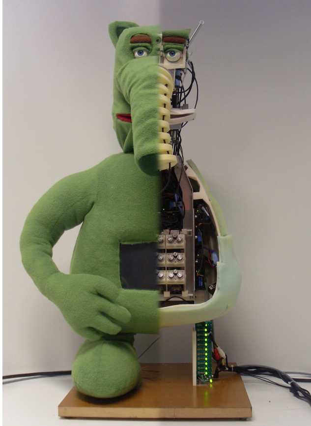
Figure 3.8: The triple layered protection covering the internal mechatronics of the prototype Probo: ABS covers, PUR foam, fur jacket.
