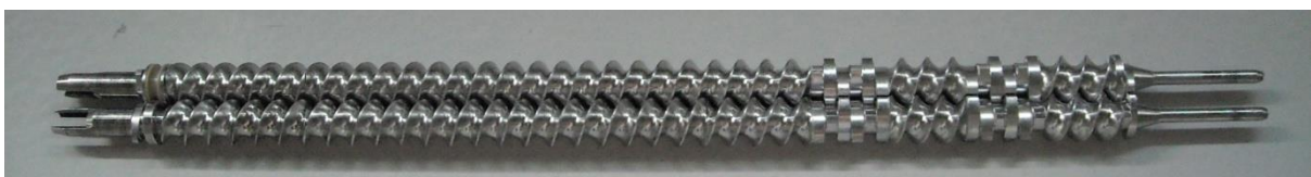
Figure 7.1. Screw configuration of the twin screws.
