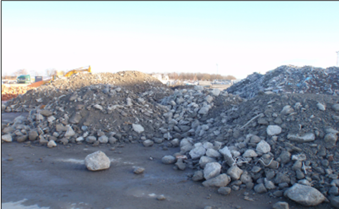
Figure 10.9.: The 0/200 recovered concrete debris
