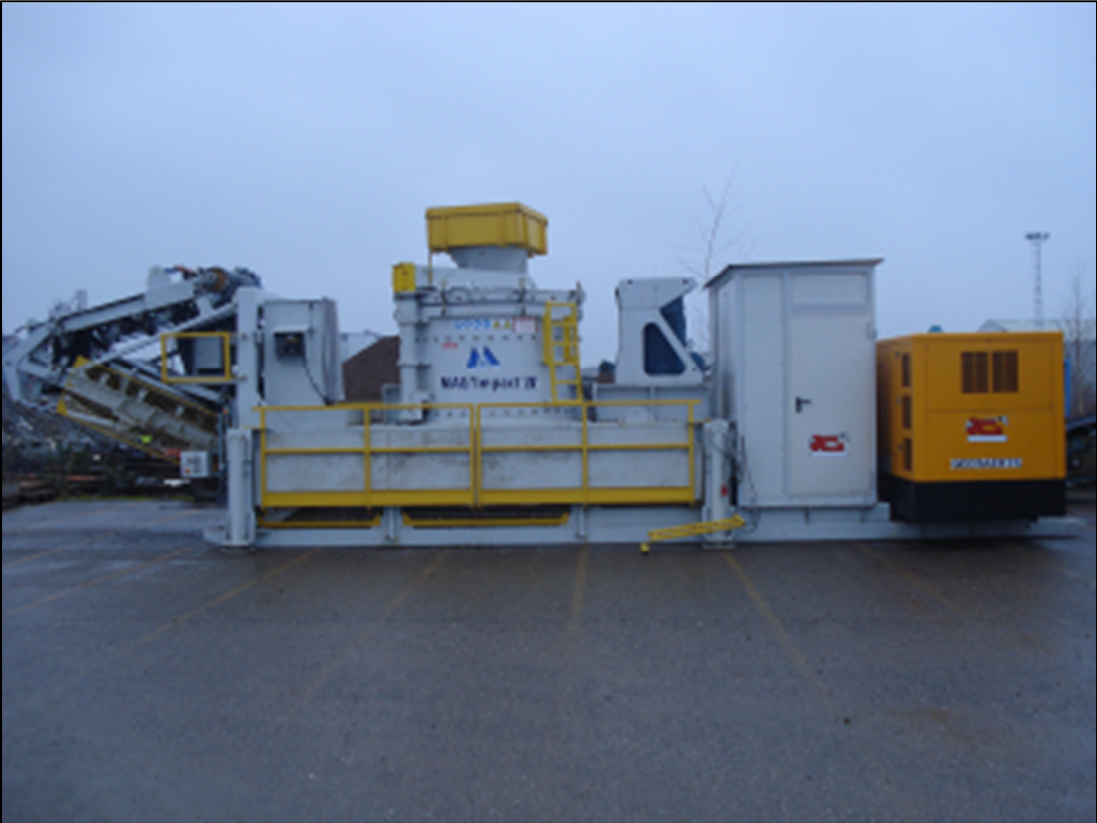
Figure 10.2.: The VSI crusher Magottaux 2400
