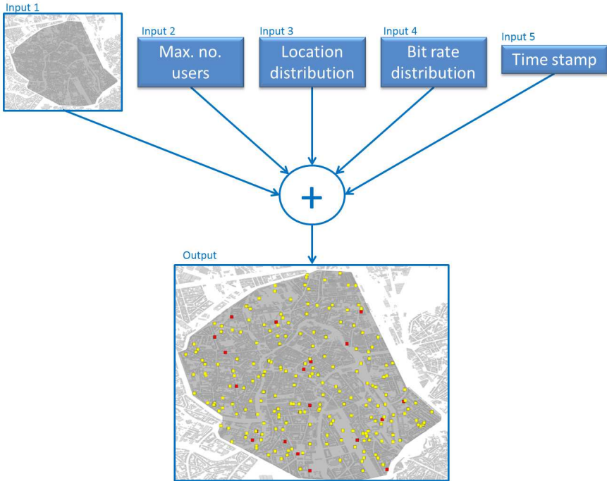
Figure 5.1: Schematic for generating realistic traffic (yellow squares in output = users requiring 64 kbps, pink squares in output = users requiring 1 Mbps).
