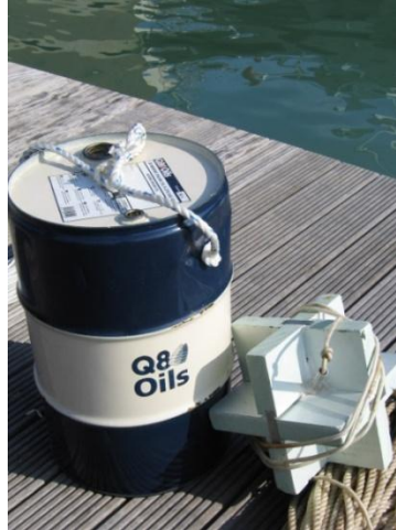
FIGURE 2-15: LEFT THE OIL BARREL, RIGHT THE ACOUSTIC REFLECTOR USED DURING THE TESTS. THE DIMENSIONS OF THE REFLECTOR ARE 20X20X20 CM, THE OIL BARREL IS APPROXIMATELY 50 CM HIGH.
