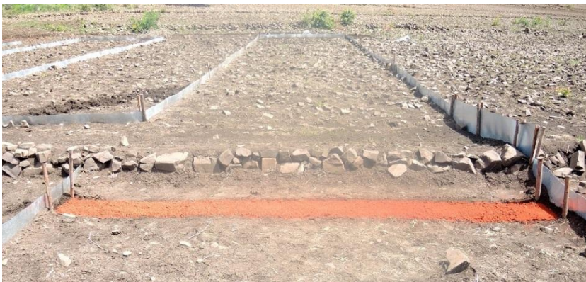
Figure 4. Overview of the erosion site (top image), and the tracer experiment (colored tracer stripe (iron oxides)) carried out at the cumulative hill slope plot (bottom image).
