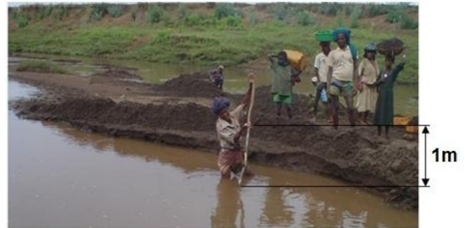
Figure 8. Thickness of deposits in the river bed in the sand mining area (after Abate et al. (2015)).
