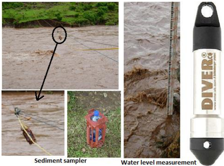
Figure 2. Details of a typical monitoring station installation at Wanzaye (Gumara River) site
