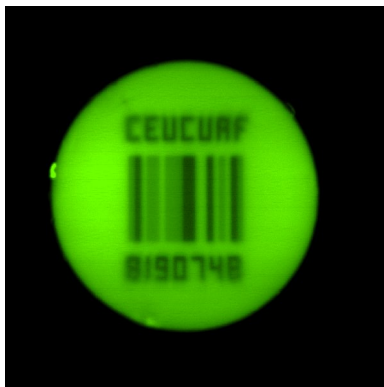
Figure 4.13: Spatial selective photobleaching. Confocal image of a 28 \mu\text{m} diameter fluorescent microsphere with a bleached barcode and an alphanumeric code.
