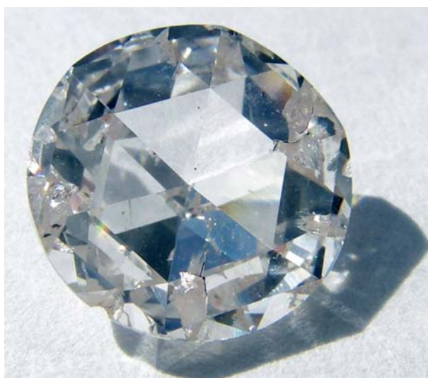
Figure 9.5: A synthetic diamond created by Apollo Diamond using a patented chemical vapour deposition process. It is 8mm wide by 2mm deep † .
