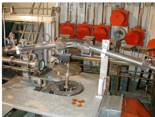
Figure 3.1: Picture of the target hall at the IRMM. The uranium target with the moderator above can be seen in the middle; the electrons are coming from the left. The orange tubes are beamstops in front of the flight paths, one beamstop is open.
