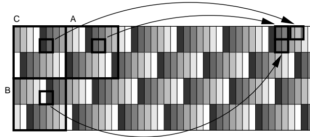
Figure 2.5: Example of a tile set in the matrix multiplication that generates conflict misses. The tiles indicated on the left occupy different memory lines that map to the same cache set (those with the same shade of grey). Cache remapping resolves this by first copying the data so that they occupy memory lines mapping to different cache sets.
