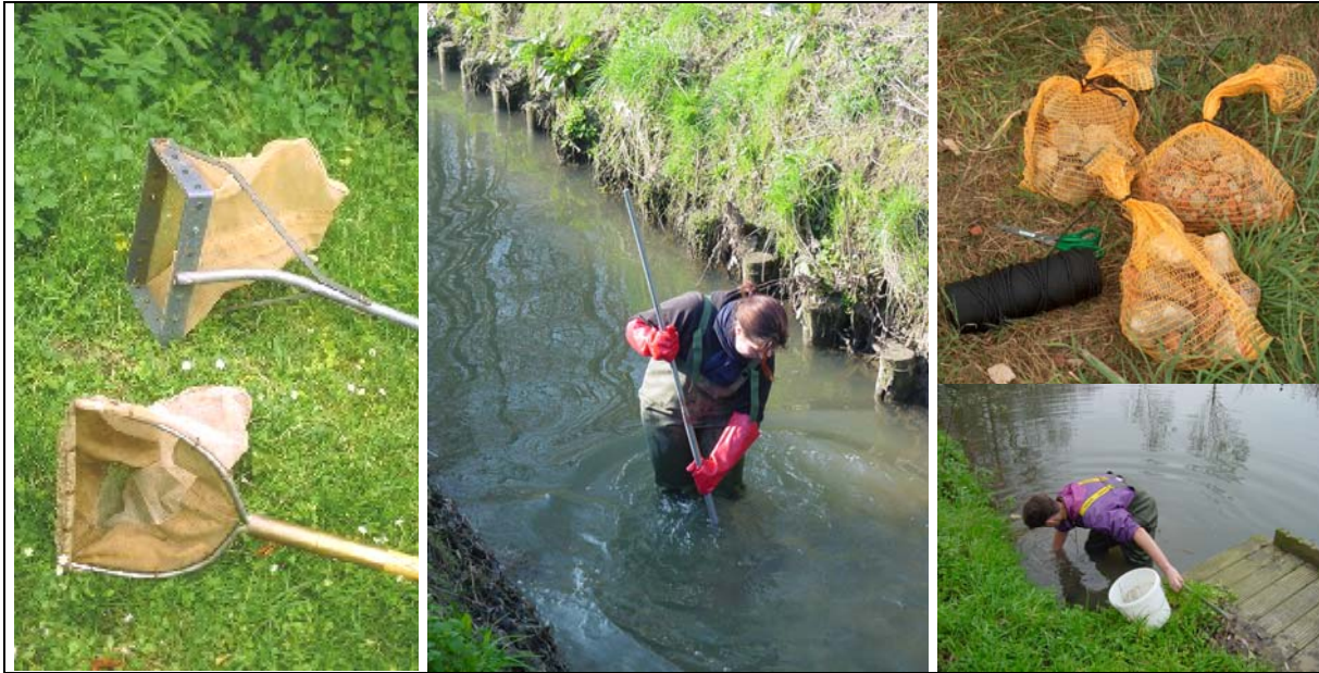
Fig. 4.7. Left and middle: handnet and kick-sampling with handnet, right: artificial substrates and retrieval of artificial substrates.
