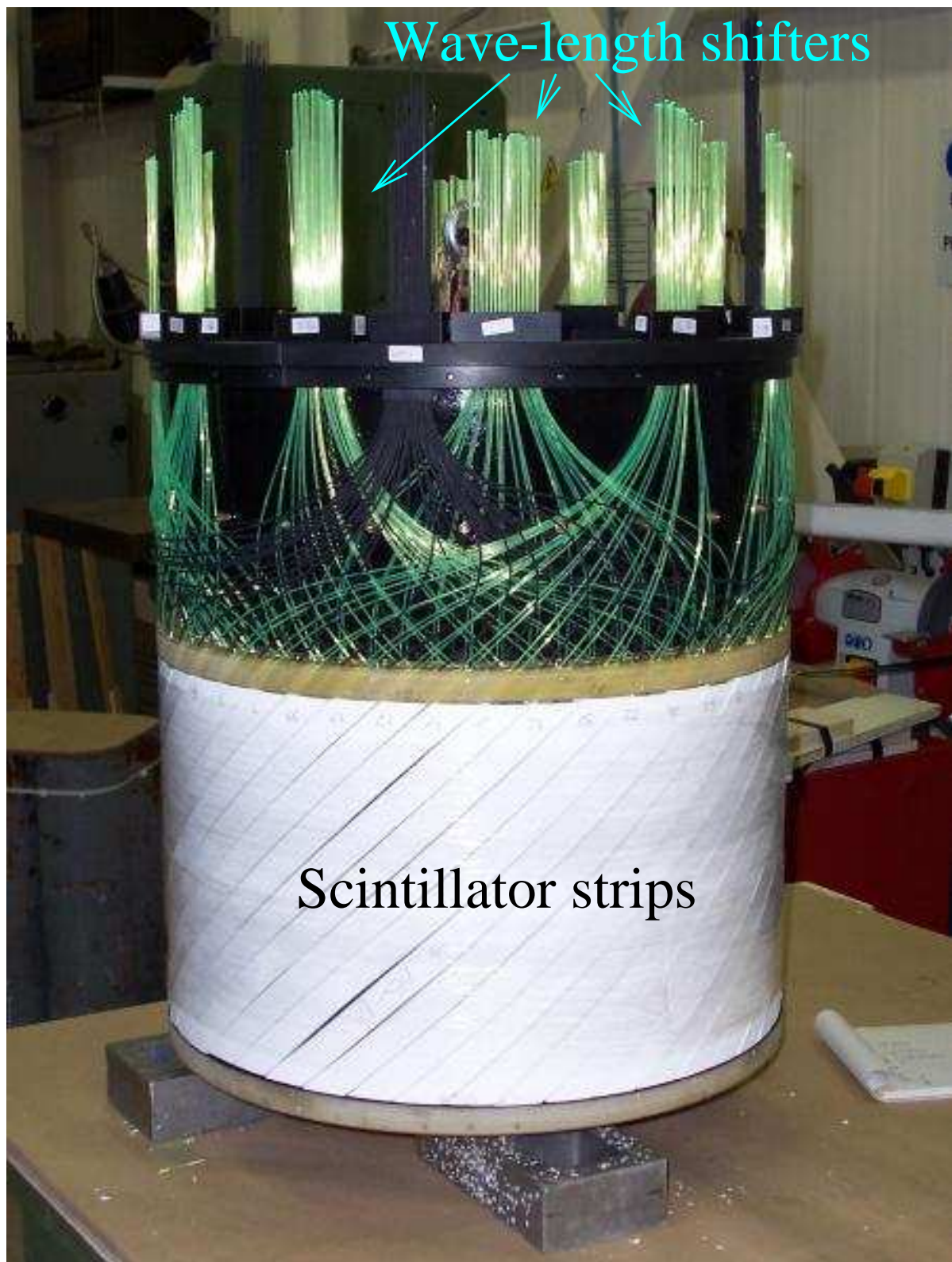
Figure 4.15: Photograph of the unfinished photon-detector. The wave-length shifters (green) and scintillator strips (white) are visible. The black fibers are light-guides for the Gain Monitoring System.
