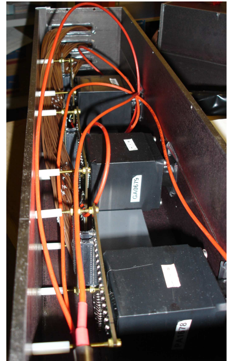
Figure 4.32: Left: the result of the magnetic shielding test. Right: a picture of 3 shielded PMTs inside a metal box.
