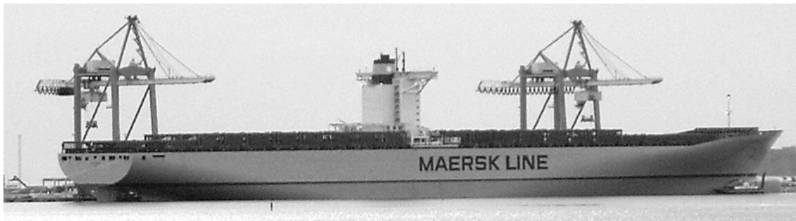
Figure 1.1. Emma Maersk, the largest container carrier ever built, having a capacity of 11000 TEU, started sailing in September 2006.
