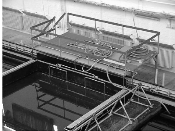
Figure 4.5. Flanders Hydraulics Research shallow water tank: mud reservoir with pump system.
