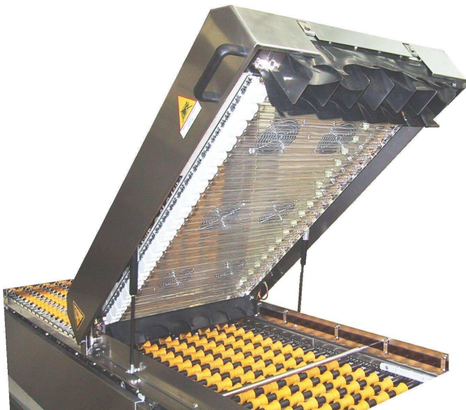
Figure 5.1: MOBA UV-disinfection unit linked to a MOBA double roller conveyer belt.
