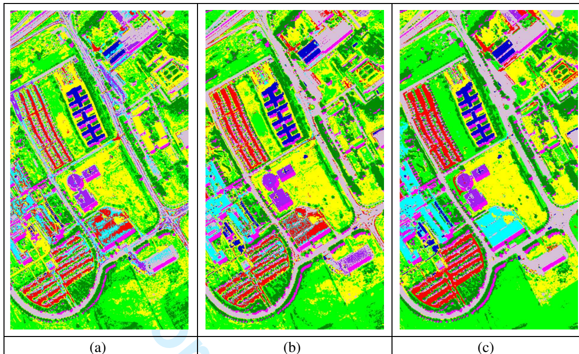
Fig. 8. Classification maps for the Pavia University image: (a) The raw hyperspectral image, (b) DMPs, and (c) GDMPs.
