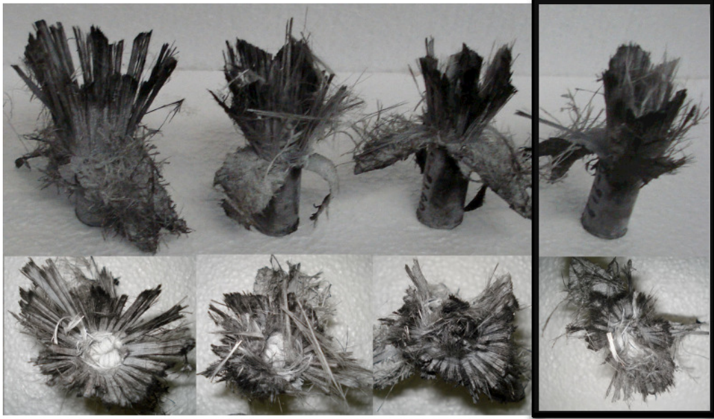
Figure 7: Tube A 60 specimens for a charge of 6g. The highlighted specimen is the one crushed asymmetrically in comparison with the rest of the specimens
