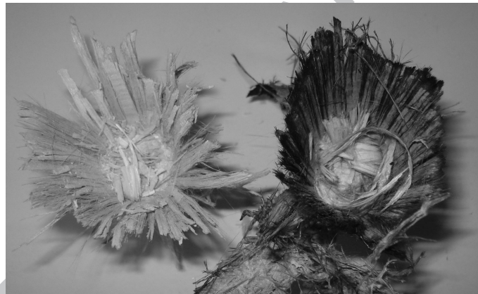
Figure 9: The specimen failure under dynamic(left) and impulsive(right) loading
