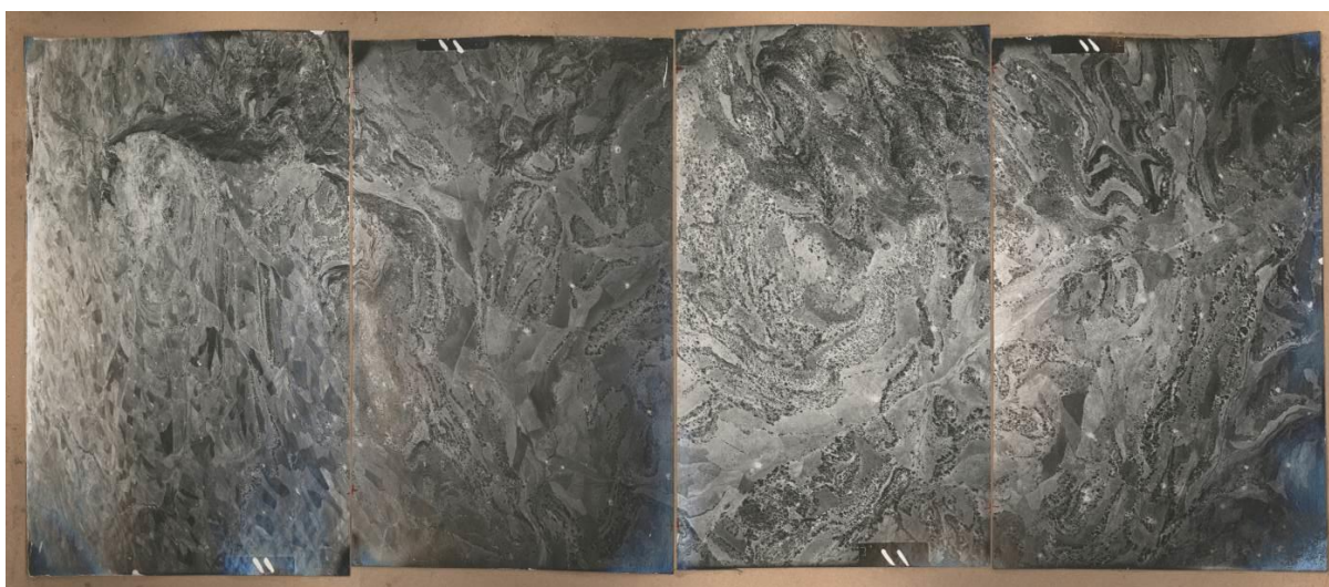
Fig. 1. An example of a set of four photographs comprising – from left to right – high oblique; low oblique; near-vertical; and low oblique exposures in a fan configuration covering an area east of Quiha in Northern Ethiopia. Date: 1935-12-16; Photo number Mai Dolo 11-2-37; centre of the vertical photo at 13.46574°N, 39.59906°E. © EMA. Width of the conformably oriented fan configuration is 36 cm on hardboard tile and 6.24 km on the terrain. Permanent farmland boundaries are clearly visible, as well as bushland that occupies structurally determined scarps. Bright dots correspond to threshing floors. The photographs cover part of the eastern edge of the Ethiopian plateau at approx. 2350 m a.s.l. Besides a dolerite sill (at left) and structural geomorphological elements (at right), the major WSW-NNE trail used by camel caravans on their way to the Arho salt plains in the Rift Valley (Afar Triangle) [43] assisted in relocating the historical AP.
