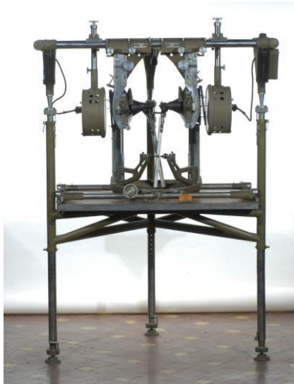
Fig. 7. The transportable Stereosimplex stereo-plotting instrument, which was based on optical-mechanical projection, designed by Santoni and built by Officine Galileo. [Source: 44, 45].
