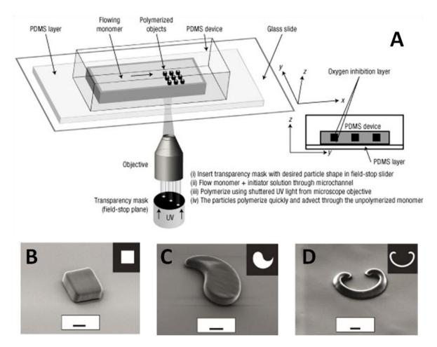
Fig. 24. (A) Schematic representation of the flow lithography technique. The device is composed of a single PDMS channel where monomer-photoinitiator solution flows. Particles are obtained by onflight fast curing. (B-D) The obtained non-spherical particles by using different UV masks. Each scale bar represents 10  $\mu$ m. Adapted from [260] with permission. Copyright 2006 Nature Publishing Group.
