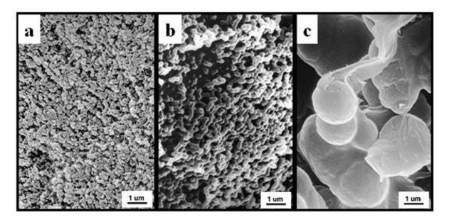
Fig. 2. Scanning electron microscopy (SEM) images from surface of EGDMA-GMA (24%-%16) beads prepared by using different porogens at 60% ratio: (a) toluene (good solvent), (b) dodecanol (nonsolvent), (c) PS solution in toluene (polymeric porogen, 50000 g/mol, 15%). From left to right, pore size increases and total surface area decreases. Reproduced from [2] with permission. Copyright 2005 Wiley-VCH Verlag GmbH & Co. KGaA.
