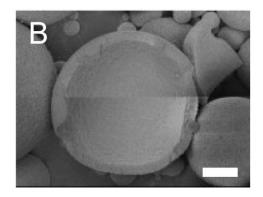
Fig. 3. (A) Porous and (B) hollow porous particles prepared by aqueous suspension polymerization, utilizing water as the porogen with the aid of various monomer soluble surfactants. Monomer soluble surfactants captured water from the continuous phase, resulting in the hollow and/or porous structure. The hollow core only formed with specific surfactants. Scale bars indicate 10  $\mu$ m. Adapted from [30] with permission. Copyright 2007 Elsevier.
