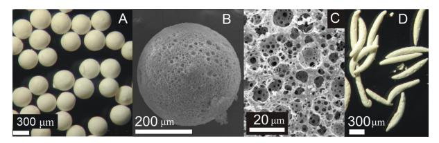
Fig. 20. Uniform poly(HIPE) beads and rods prepared via a tubing-needle microfluidic device. (A) Light microscopy image of beads showing monodispersity, (B) SEM image of a single poly(HIPE) bead, (C) SEM surface close-up of a poly(HIPE) bead. Pores are reaching up to 15  $\mu$ m and all interconnected, (D) Poly(HIPE) rods prepared from a more viscous HIPE mixture. Adapted from [9] with permission. Copyright 2009 American Chemical Society.
