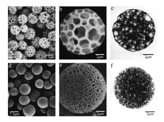
Fig. 11. SEM (A, B, D, E) and TEM (C, F) images of hollow core, porous shell ("cage-like") particles prepared by a combination of Pickering emulsion approach and  $\gamma$ -ray polymerization of additional monomer that are swelling these seeds (see Fig. 12 for the mechanism). (A-C) PMMA, (D-F) poly(vinylacetate). Adapted from [107] with permission. Copyright 2005 American Chemical Society.
