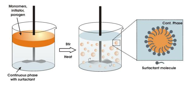
Fig. 1. Basic depiction of the suspension polymerization technique.
