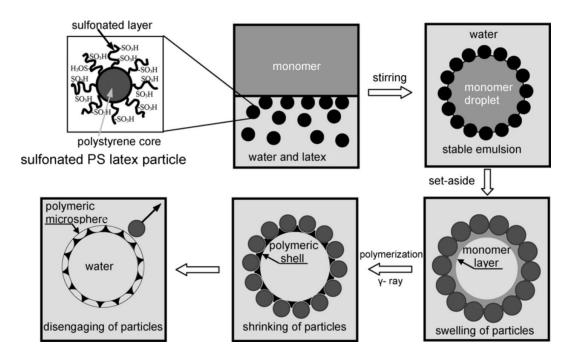
Fig. 12. Mechanism of the formation of "cage-like" particles shown in Fig. 11. Adapted from [107] with permission. Copyright 2005 American Chemical Society.
