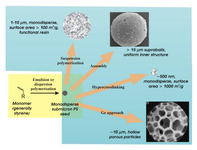
Fig. 13. Overview of multistage approaches with the monomer styrene as an example. In the first stage (yellow background), monodisperse submicron seeds are prepared. The second stage (blue background) can be either suspension polymerization to obtain larger and porous particles, or assembly to obtain supraballs, or hypercrosslinking to obtain very high surface areas or a combination of assembly and polymerization (Ge approach) to obtain cage-like particles.
