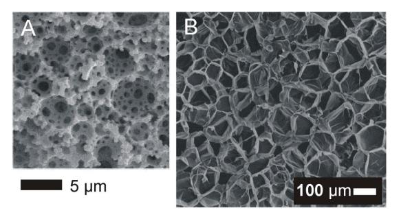
Fig. 4. The surface of (A) a poly(HIPE) bead [36] and (B) a water expanded PS bead [40] both prepared by suspension polymerization using water as the porogen. While the largest pore is only  $\sim$ 5 µm for the poly(HIPE) bead, the water expanded PS bead possesses pores as large as 100 µm. Adapted from [36, 40] with permission. Copyright 2002 Elsevier; Copyright 1999 Elsevier.
