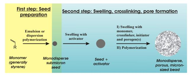
Fig. 8. Schematic description of seeded suspension polymerization for obtaining porous particles. In the first stage, submicron seeds are prepared from styrene by emulsion or dispersion polymerization. In the second stage, that is being suspension polymerization, seeds are first swollen with an activator (i.e. dibutyl phthalate) and then swollen with new monomer, crosslinker, initiator and porogens. Polymerization results in larger, porous and monodisperse particles.
