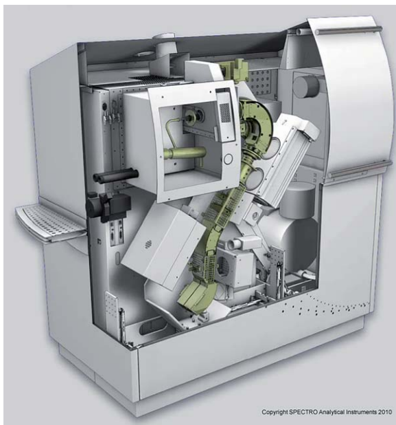
Fig. 19 Schematic drawing of the Spectro MS (Spectro) (source: Spectro Analytical Instruments).
