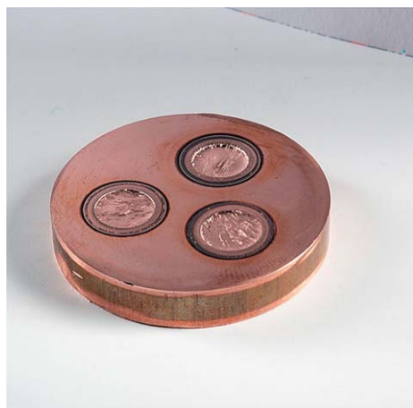
Fig. 14 Crater from 3 different sputtering events in the GD source of the Element GD (sample: BCR copper standard CRM 075).
