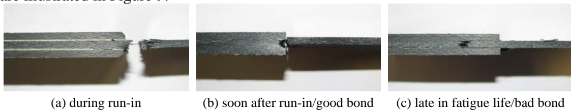
Figure 9 Overview of the occurring tab failures during fatigue experiments
