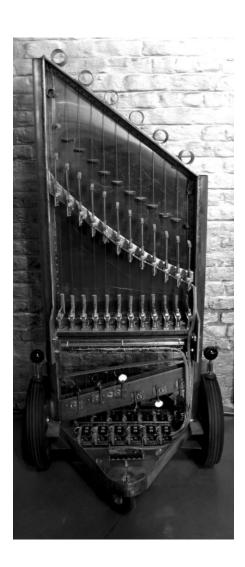
two electromagnets, driven by a two-phase signal on opposite sides of the string. The Ebow is an electronic device that generates an electromagnetic field, commonly used to move a string, such as on an electric guitar (Raes 2010d).
