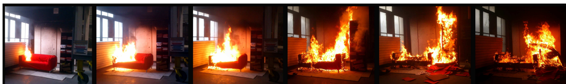
Figure 6- Sequence of images of flame spread and burning in Test1 (Lab).
