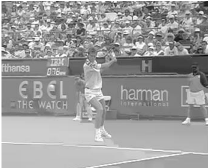
(b) Spatial drift in intra-coded picture (Stefan, frame 15, transcoded using OL, QP_1 = 22 , QP_2 = 28 )
