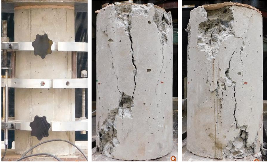
Figure 3.8: Failure modes of the concrete cylinder.
