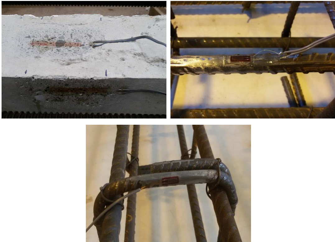
Figure 3.14: Strain gauges bonded to concrete and longitudinal tensile and transverse reinforcement before being protected.
