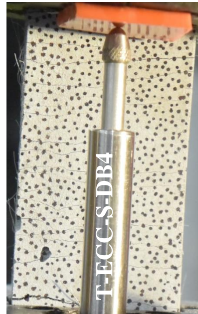
(b) 4% strain Crack number = 15 Mean crack width = 47 \mu\text{m} Max crack width = 150 \mu\text{m} Min crack width = 20 \mu\text{m}
