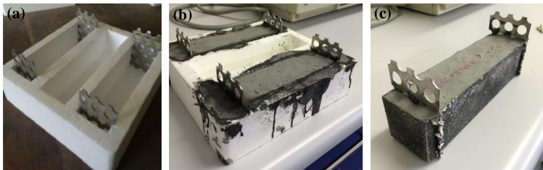
Figure 3.4: (a) Polystyrene moulds and electrodes; (b) ECC prismatic samples after casting; and (c) an example of a prismatic ECC sample after demoulding.
