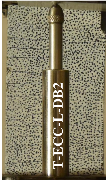
(c) 4% strain Crack number = 11 Mean crack width = 60 \mu\text{m} Max crack width = 110 \mu\text{m} Min crack width = 20 \mu\text{m}
