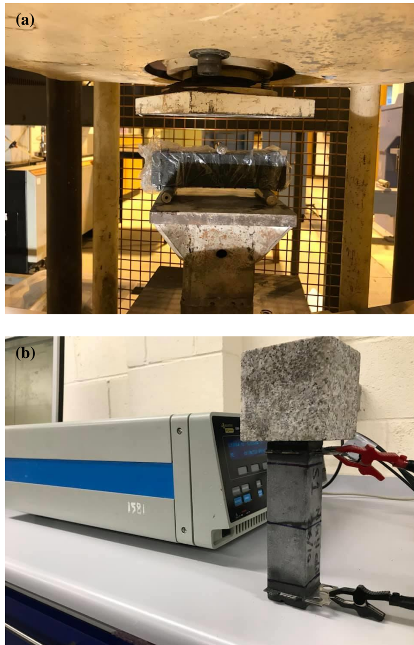
Figure 3.12: (a) Test setup for precracking the sample and (b) electrical measurements of the single-crack sample.
