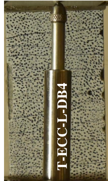
(d) 4.4% strain Crack number = 12 Mean crack width = 103 \mu\text{m} Max crack width = 160 \mu\text{m} Min crack width = 70 \mu\text{m}
