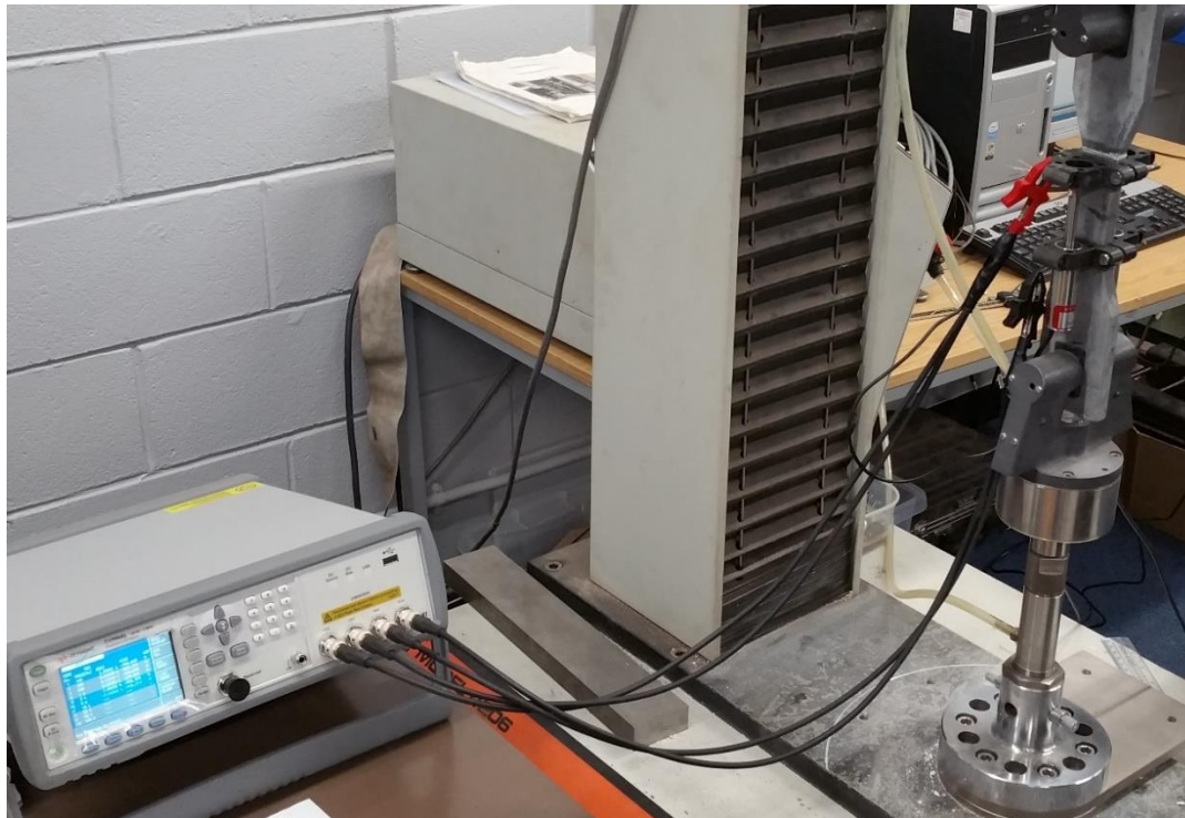
Figure 3.10: Piezo-impedance test setup displaying the LCR meter on the left and a specimen under testing on the right.
