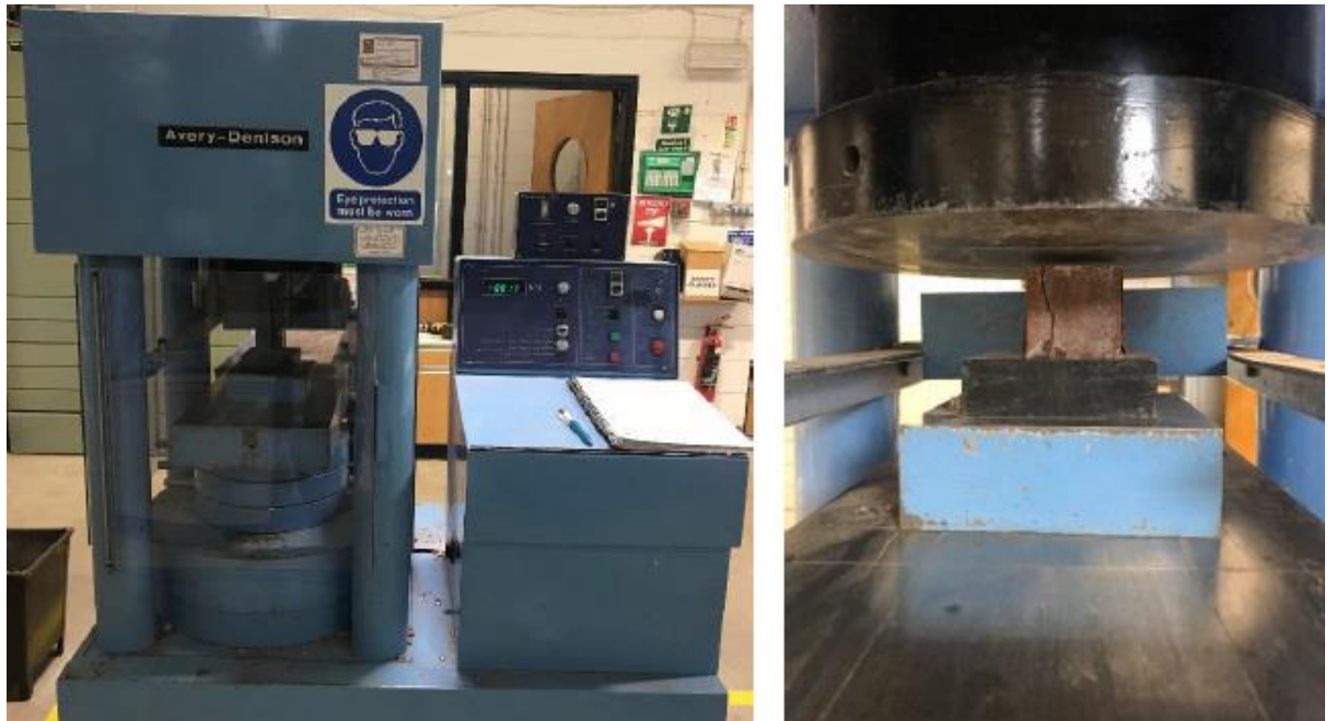
Figure 3.7: Experimental setup for the compression tests.
