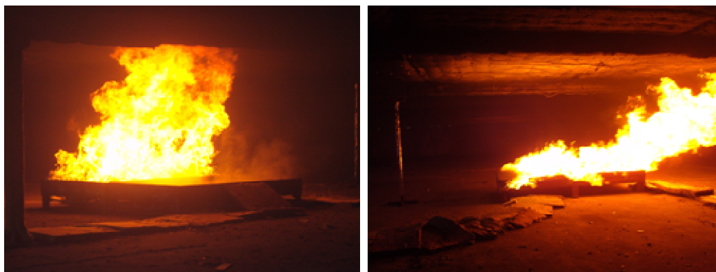
Figure 3. Pictures of a 4 MW fire in the OOOOO (left) and XXOXX (right) configuration. Extraction rate = 200000 \text{ m}^3/\text{h} .
