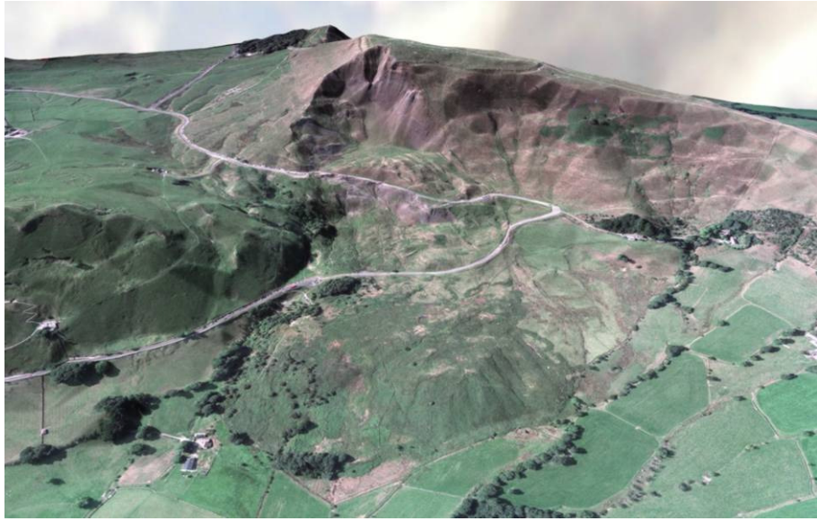
Fig. 12. A realistic impression of the Mam Tor landslide, created through draping an orthophoto over a DEM, both obtained from the 1999 images.
