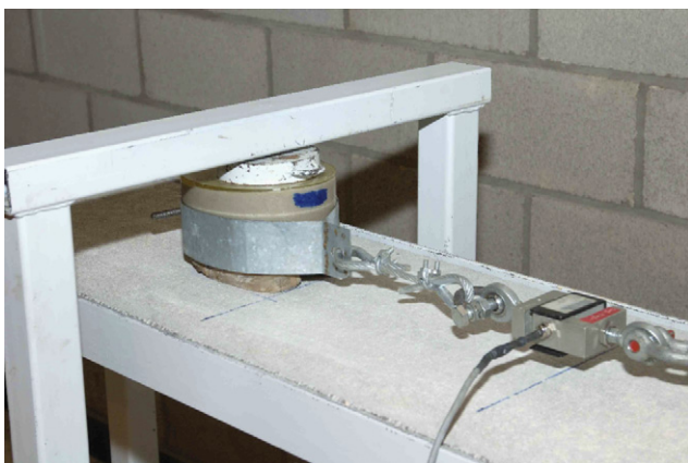
Fig. 3. Detail of claw model on concrete panel, load cell, dragging mechanism and sub frame to transfer normal load
