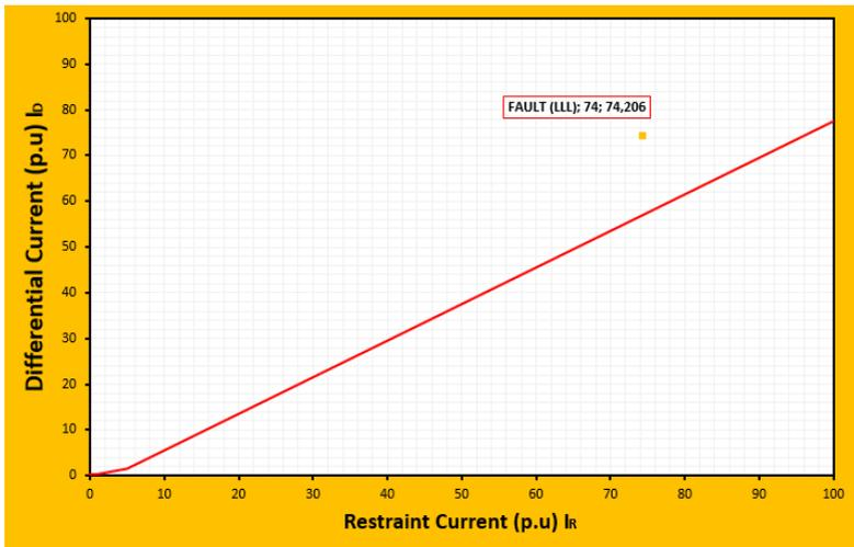
**Gambar 4.5** Kurva Operasi Rele Diferensial Gangguan Internal Primer
