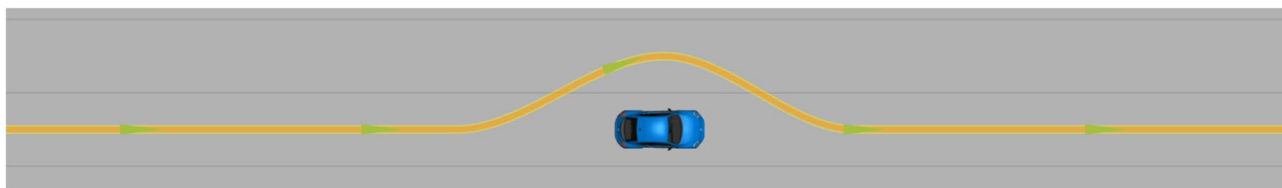
Fig. 6 Double lane change maneuver used for verification of the implemented control concept. Yellow line represents the translational path of the target trajectory used
