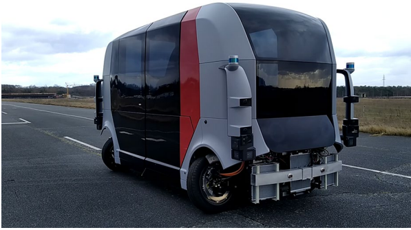
Fig. 1 Sideways parking of UNICARagil vehicle “autoSHUTTLE” with 90° wheel steering angle on all wheels, utilizing the independent dynamics modules
